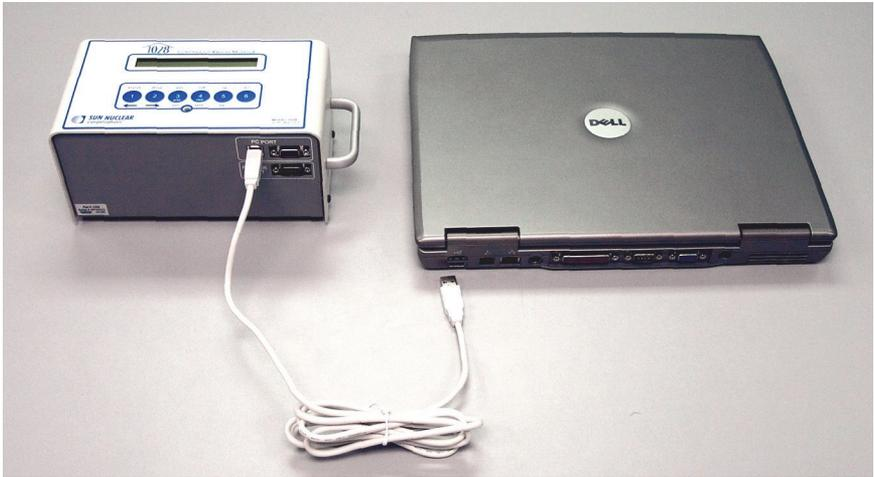
Figure 15. USB Connection to a Computer
