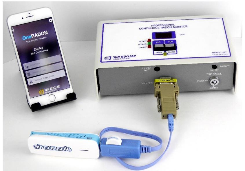
Data will now transfer automatically to the *OneRADON* app. After transfer the Spinner will disappear followed by Pop up boxes for input of Serial number, Cal date, correction factor, Start dates to promote this missing information to the reporting. Correction factors will automatically calculate to the averages.
